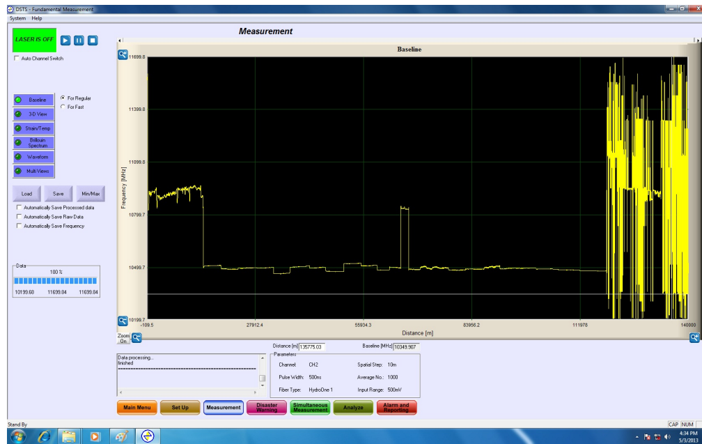
Fig. 9 Brillouin frequency shifts along the fiber, loop back point located at 66.6-km (the high reflectance event).
