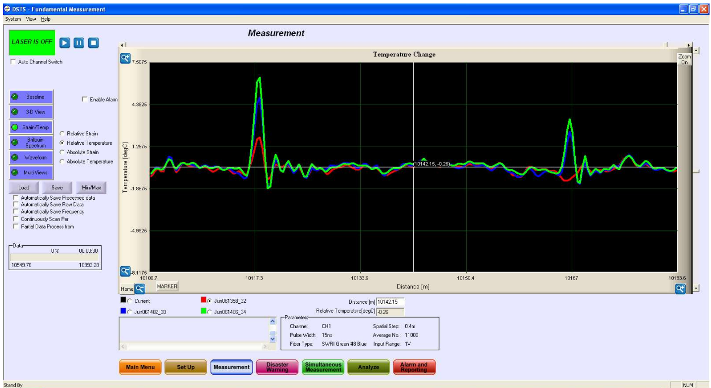
Fig. 12. Leakage volume of 2.187 gal has been detected in 1 minute after a leak happened, shown as the red peak at 10,118.06 m.
