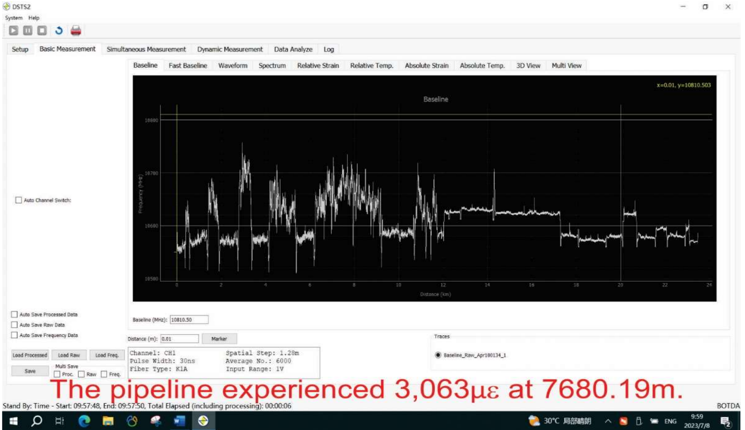
Fig. 9. Pipe experienced 3,063\mu\epsilon during winter from November 2022 when the pipeline was installed to April 2023 when the soil was still frozen.
