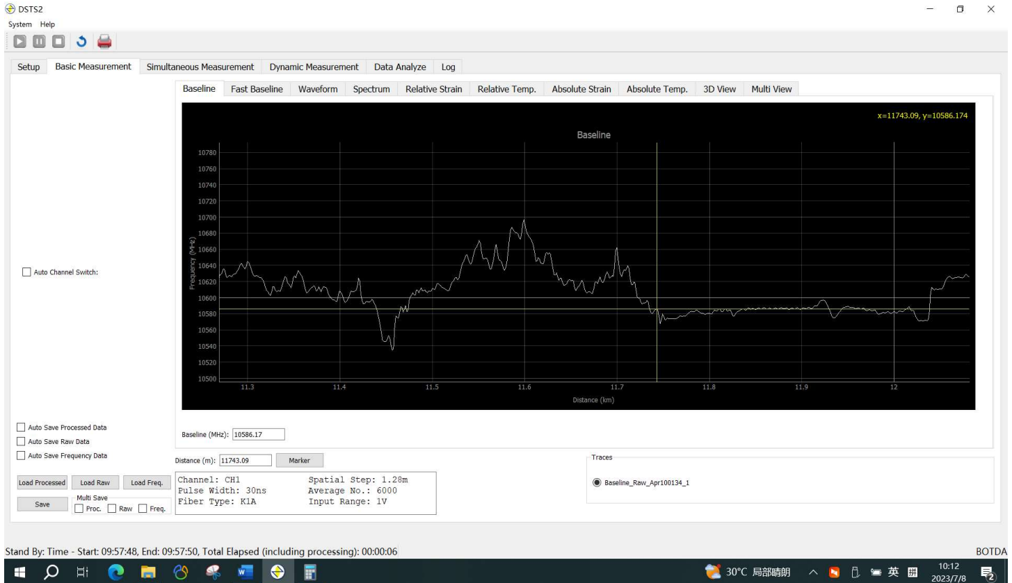
Fig. 5. Loosed and tight-buffer optical cables were connected at 11,743.10m.
