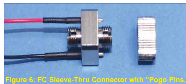
Figure 5: FC Sleeve-Thru Connector with "Pogo Pins."
