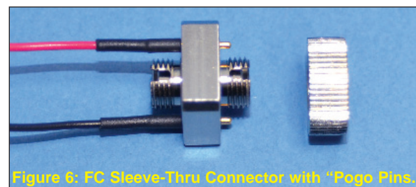
Figure 5: FC Sleeve-Thru Connector with "Pogo Pins."
