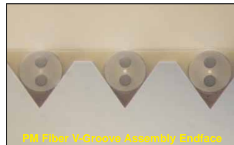
8 Channel PM Fiber Pigtailed V-Groove Array
