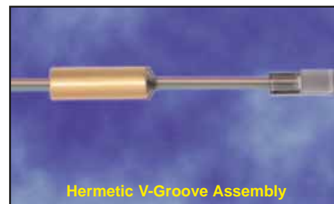
PM Fiber V-Groove Assembly Endface
