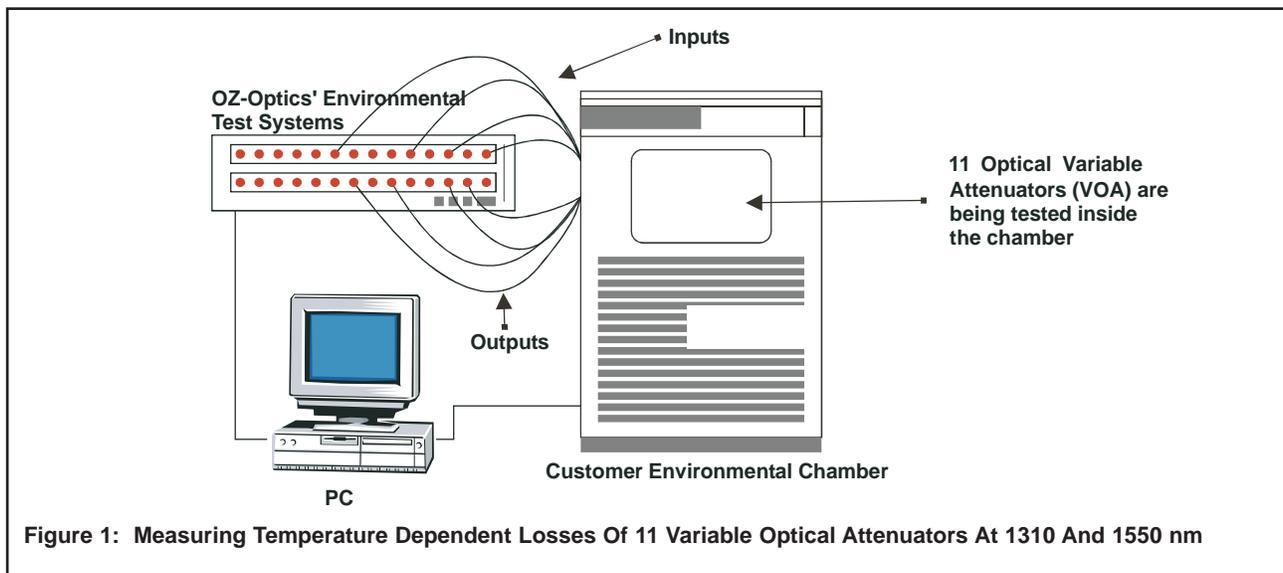
Figure 1: Measuring Temperature Dependent Losses Of 11 Variable Optical Attenuators At 1310 And 1550 nm
