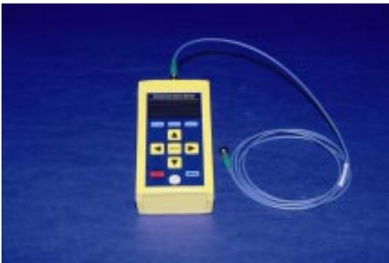
Polarization Extinction Ratio Meter
