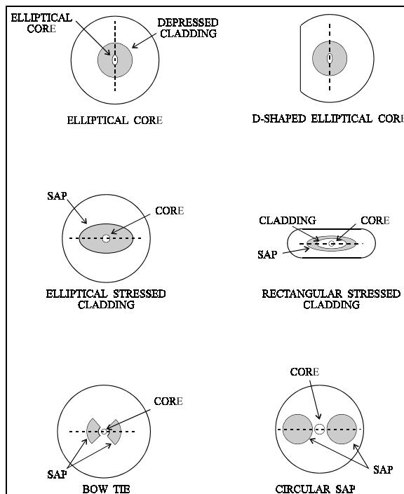
**Figure 2:** Examples of polarization preserving fiber core structures.
