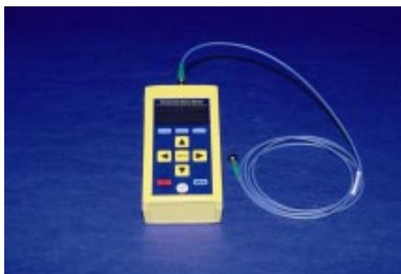
Polarization Extinction Ratio Meter
