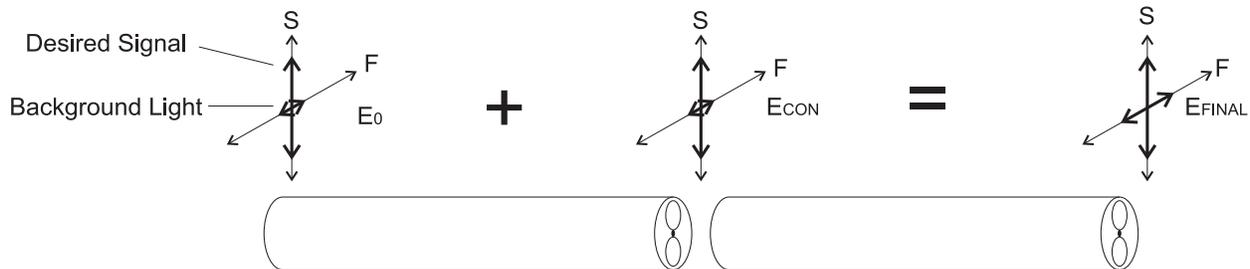
Figure 4: Degradation of Polarization at a Connection
